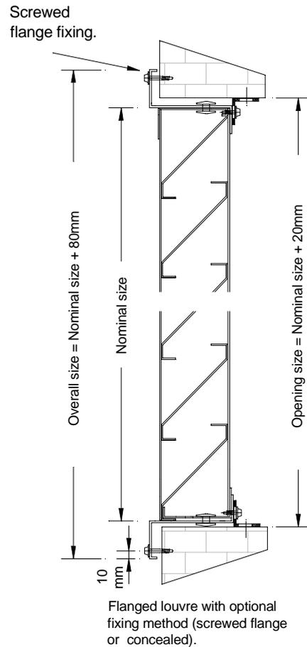
AHE 'LOUVRE-LOCK'<sup>®</sup> External louvres are manufactured from plastic coated galvanised steel (ALUZINK) using a unique interlocking assembly process. Specially developed for use on mechanical fresh air input and exhaust air systems, these products are ideally suited for incorporating into new and existing buildings. Available in a wide range of colours to suit most new modern building styles or alternatively in plain galvanised finish where aesthetic appearance is less importance.
