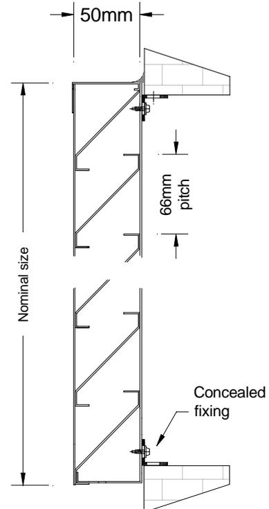
Surface mounted louvre with concealed (internal) fixings for high security application.
